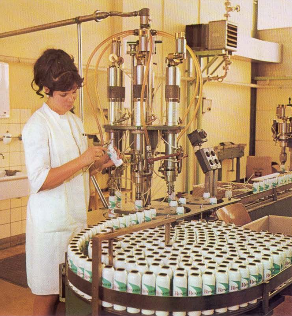
(LEFT) The final stages in the production of Rexona deodorant at the Elida-Gibbs factory in Hamburg. The aerosol packs are filled and pressurised.
